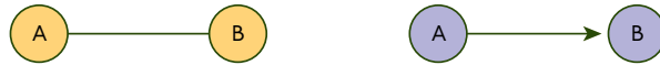
Figure 1.4: Diagrams representing graphs with vertex set V = \{A, B\} and edge set E = \{(A, B)\} . The diagram at left is for an undirected graph, while the one at right shows a directed graph. Thus the arrow on the right represents the ordered pair (A, B) .
